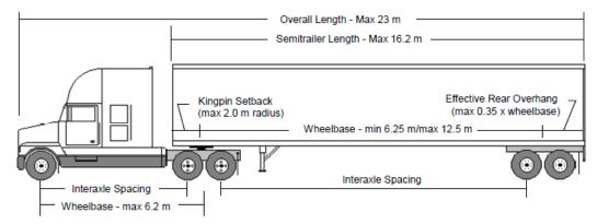
The new authorization grants that the truck tractor wheelbase can be increased up to 7.2 m in a tandem drive truck tractor-semi-trailer configuration, provided the wheelbase of the semi-trailer is reduced in accordance with the following table:
