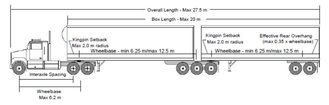
Appendix B of the CTR provides a maximum wheelbase of 6.2 m for tandem drive truck tractors. Appendix G of the CTR provides a maximum wheelbase of 12.5 m for each semi-trailer.
